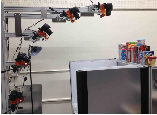
Fig. 3. Side view of all Carmines mounted to respective Canon T3s, pointed at the Ortery Photobench. The dimensions of the Photobench are 31" D x 26"H x 26" W.
